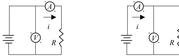
Figure 7 – Two alternative options to realize the ideal solution of an exemplary measurement problem.
