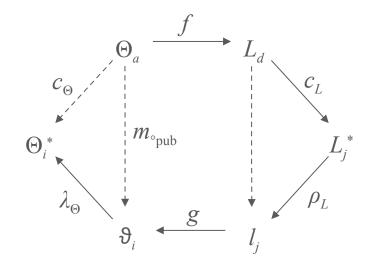
The result of measurement is  $\Theta_a = \vartheta_i \circ \text{pub}$  (e.g.,  $\Theta_a = 20 \circ \text{C}$ ) i.e.,  $c_{\Theta}(\Theta_a) = \Theta_i^*$  (e.g., value-of( $\Theta_a$ ) = 20 °C) i.e.,  $m_{\circ \text{pub}}(\Theta_a) = \vartheta_i$  (e.g., value-in-°C-of( $\Theta_a$ ) = 20)
