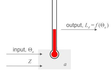
The limited selectivity of the instrument reduces the objectivity of the information produced by the measurement
