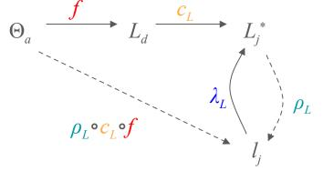
According to this simple model, pre-measurement results may convey object-related (*objective*) information A model of measurement / 2
