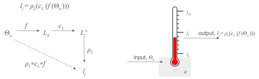
It is a sort of *private* (because *instrument-specific*) measurement, whose result is The value of  $\Theta_a$  is  $l_i$  in the scale °mydev if and only if  $\rho_L(c_L(f(\Theta_a))) = l_i$
