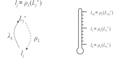
Under the hypothesis that the instrument is stable, the identifiers  $l_j$  make the comparison of results of transductions performed in different times possible
