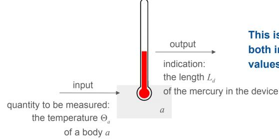
This is an empirical transduction: both input and output are physical states; values of quantities are not here yet
